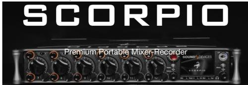
Another IBC winner, the Scorpio is a 32 channel, 36 track mixer-recorder and the most powerful product ever designed by Sound Devices. This tiny device contains 16 mic/line preamplifiers, 32 channels of Dante in and out, AES in and out, 12 analog outputs and multiple headphone outputs.
